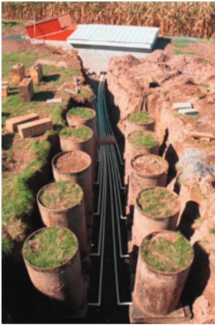
Figure 2. Zero-tension lysimeters, 0.76 m diameter and 1 or 2 m deep, at the Masser Recharge Site, Pennsylvania, operated by USDA-ARS. Water percolating out of each lysimeter is collected and automatically weighed at 30-minute intervals. Downward fluxes computed from these data are interpreted as recharge-rate estimates.
