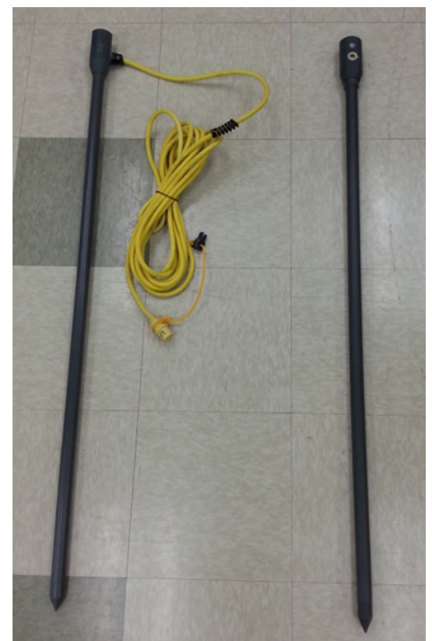
Fig. 1: One-meter long temperature probes with and without integral communication cable. Data are stored in individual embedded sensors and can be retrieved through the cable (left probe) or through a handheld reader making temporary contact with electrodes on the head of the probe. Both probes can be downloaded while submerged in water.
