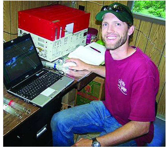
Jared Trost analyzing soil gas samples on a GC. Photo from Isanti County News , March 1, 2015.
