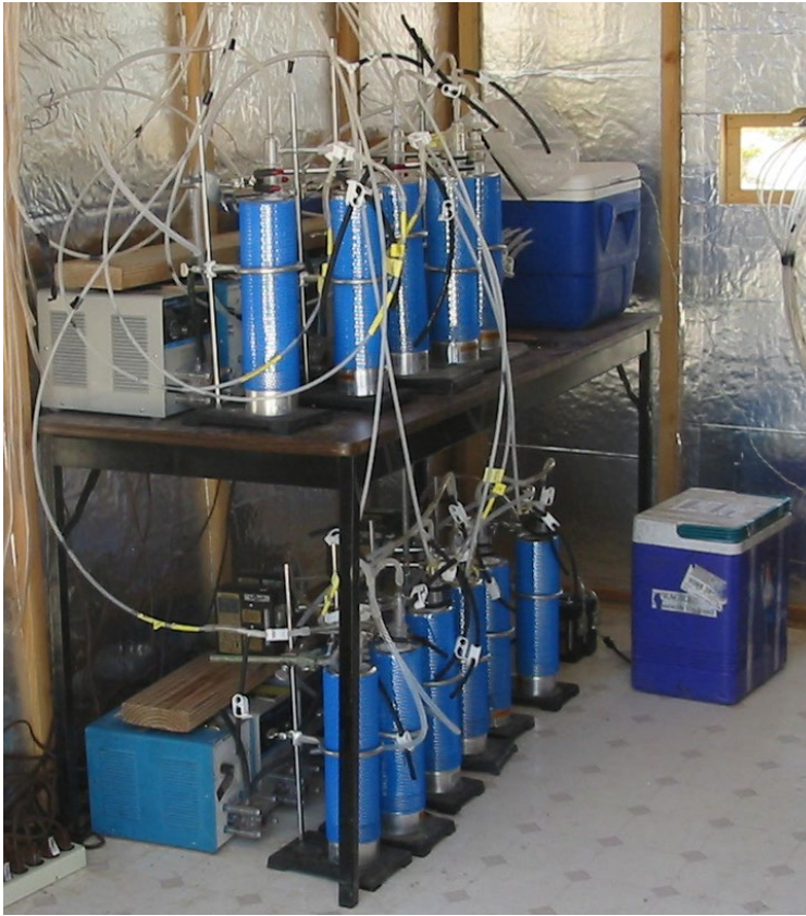
Amargosa Desert Research Site (Nov. webinar topic). Tritiated water vapor sampling from unsaturated-zone borehole #3 at the Amargosa Desert Research Site, NV. Photo by Justin Mayers, May 2004.
