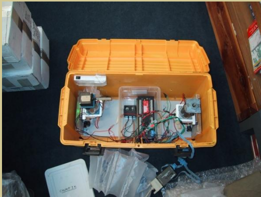
Pump setup for tracer injection
