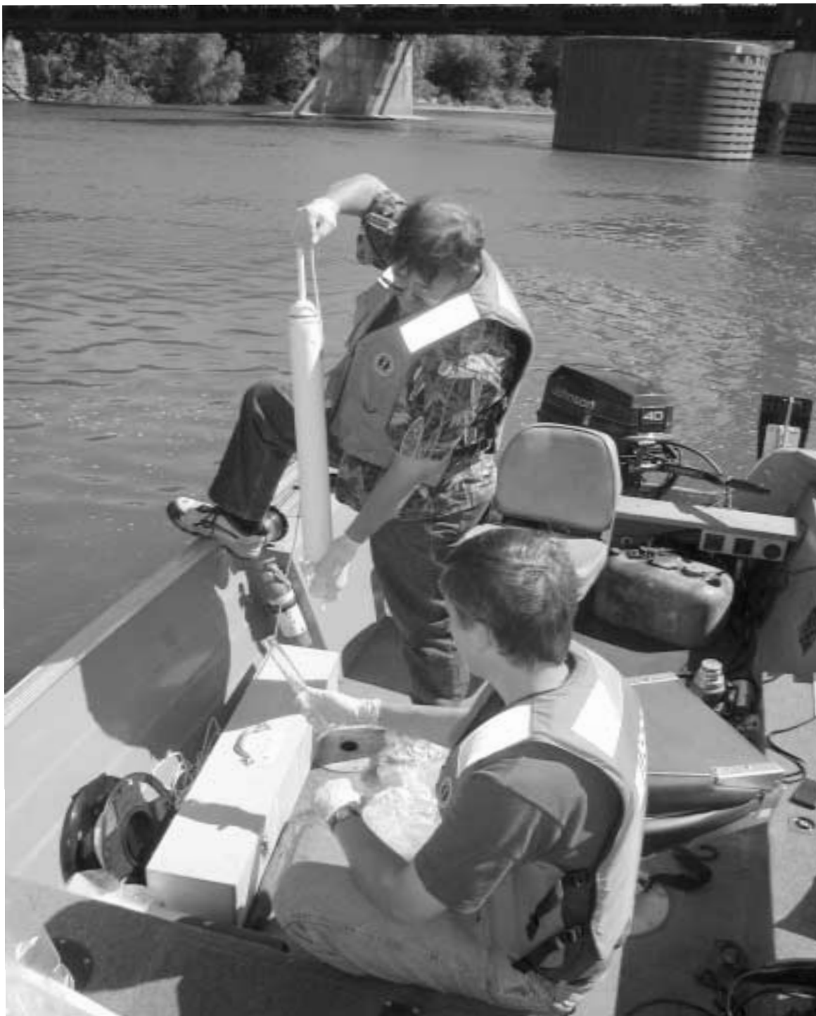
Water quality sampling with plunge sampler, August, 2002
