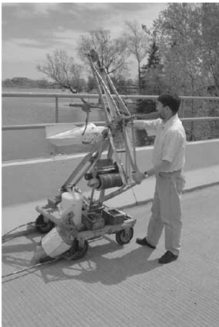
Water-quality sampling with bridge-suspended equipment.
